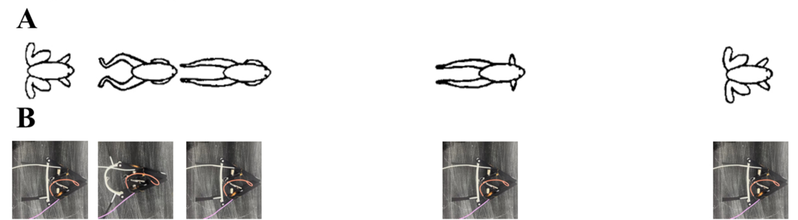
Figure 6. Comparison of swimming posture between frog and bistable robot. A) The swimming posture of a frog during a cycle [5] . B) The swimming posture of a bistable robot during a cycle
