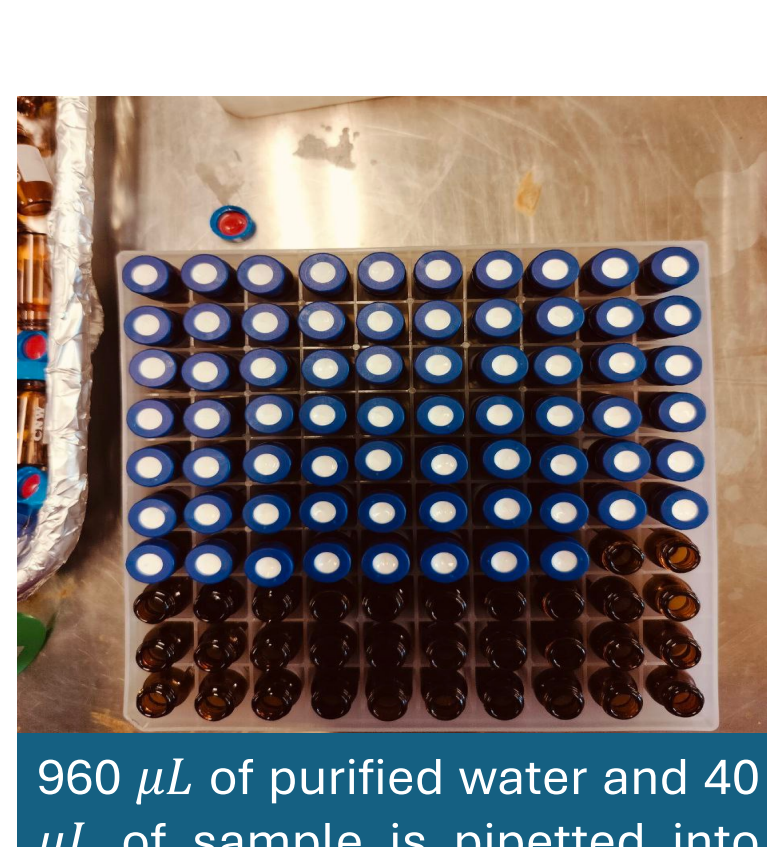
960 µL of purified water and 40 µL of sample is pipetted into each HPLC bottle for analysis.
