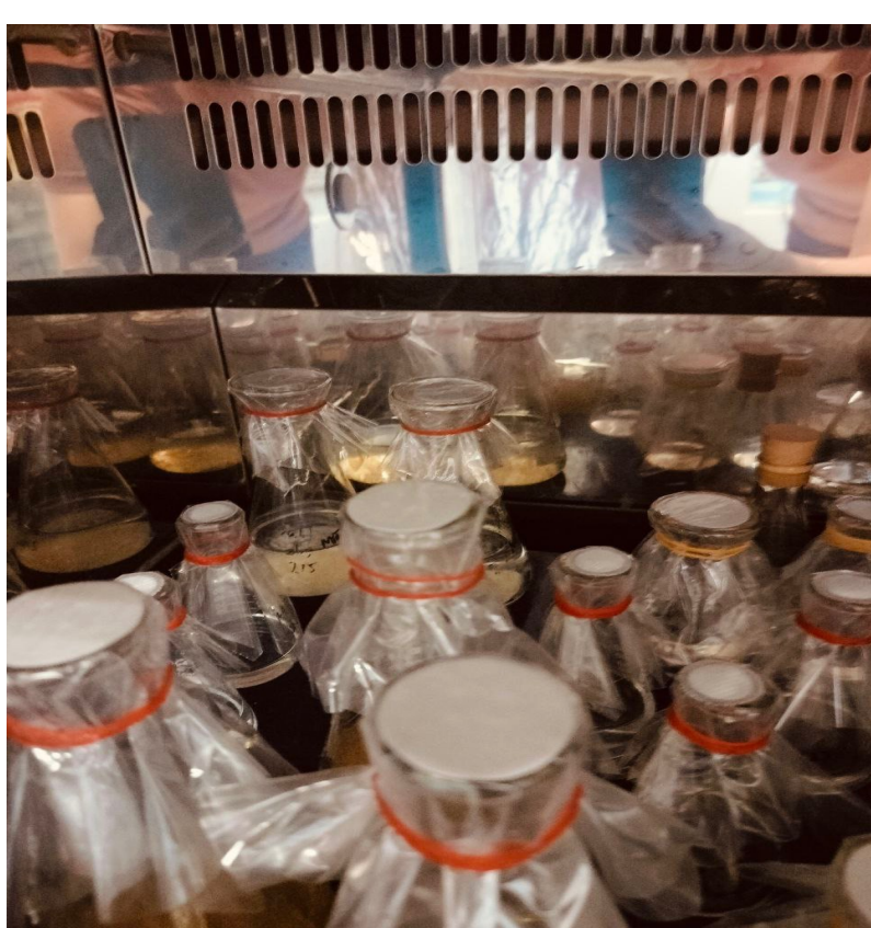
In between sampling, the flasks are stored at 30°C and 150 rpm in a rotary shaker.
