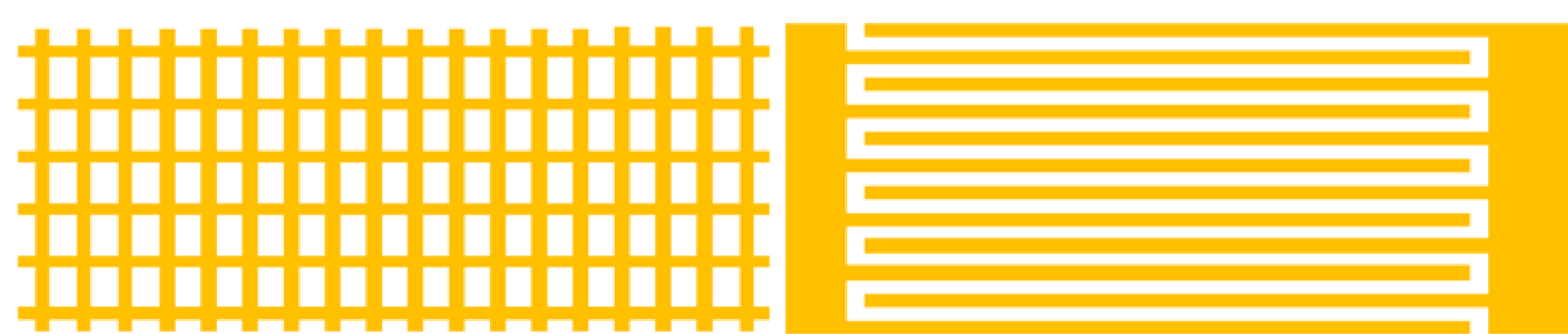
Figure 2: Patterns used on the substrate. On the left, the original pattern, on the right, the new design pattern with two electrodes (not to scale).
