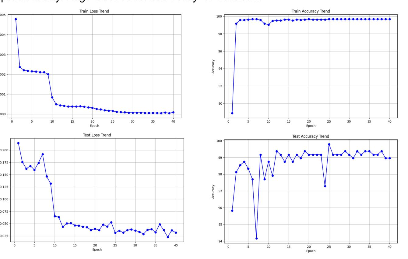
The final training results demonstrate the model's exceptional performance, with an average loss of 0.0021 and 100% accuracy on the training set, and an average loss of 0.0320 and 99% accuracy on the test set. These results indicate that the model has effectively learned and generalized well, making it highly suitable for practical applications in action recognition using DVS data.
