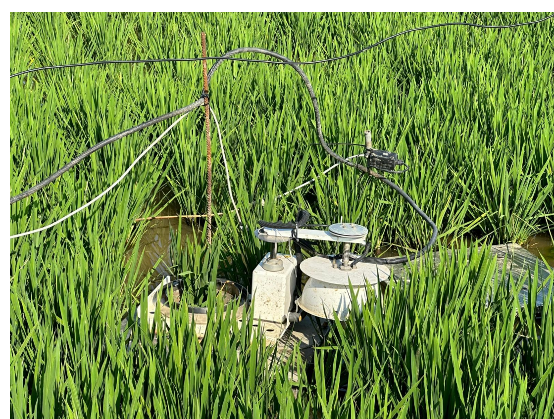
Fig 3: Picture of an open chamber device with a rice plant inside. Picture taken at the measurement site.
