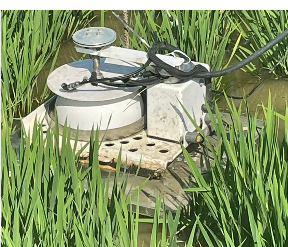
Fig 2: Picture of a closed chamber device. Picture taken at the measurement site.
