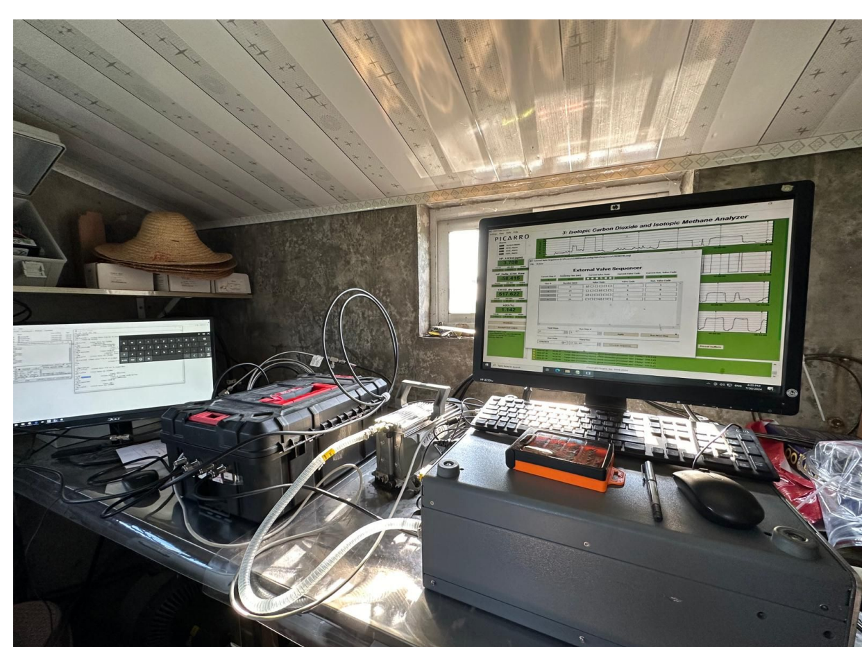
Fig 4: Picture of the Picarro G2201-i device (box under the desktop). Picture taken at the measurement site.
