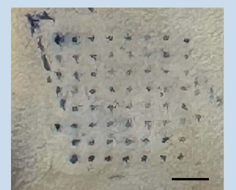
Fig. 6 Skin penetration efficiency test. (Scale bar: 2mm)
